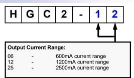
The current range represents the maximum current output available. The module output current should ideally just exceed or equal the valve selected.
