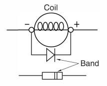
A typical diode is 1N4005 which is readily available from commercial sources. Failures of this type are not covered by our Limited Warranty.
