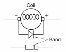
A typical diode is 1N4005 which is readily available from commercial sources. Failures of this type are not covered by our Limited Warranty.
