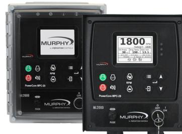
Murphy's ML2000 control panel incorporates all the power and functionality of the PowerCore® MPC-20 in a panel solution for most any engine-driven application.
