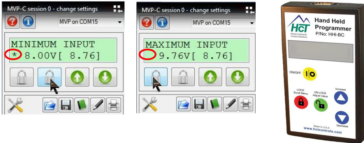
Use the up and down arrows to navigate through the parameter list. The display will show the next parameter in the list when pressed. The parameter name is on the first line and the value is on the second line. The list scrolls, stepping down from the last parameter to the first and vice-versa.
