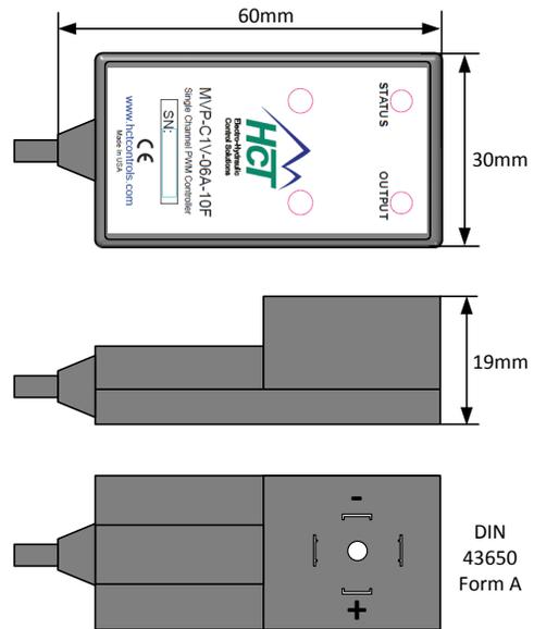
There are two indicator LEDs: STATUS and OUTPUT. The STATUS LED is green when the applied voltage is within the operating range.
