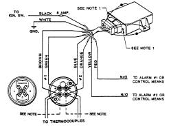
4) Single pyrometer and pyro-switch 030-058(-1)
