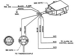
2) Dual pyrometer with pyro-switch 030-017(-1)
