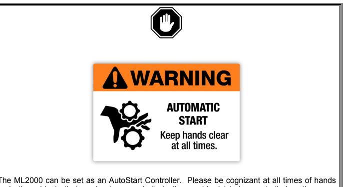
The ML2000 can be set as an AutoStart Controller. Please be cognizant at all times of hands and other objects that are in close proximity to the machine(s) being controlled as they may commence operation suddenly and without warning.
