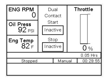
This screen displays the auto start/stop type and will also illustrate the throttling method for the auto start/stop. This screen is set to display dual contact start (floats) and throttling to max RPM.
