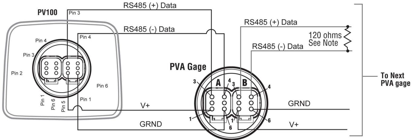
**Note:** Place Resistor between RS485+ and RS485- at end of Line on last PVA gage (included in PVJR or factory purchased panels).
