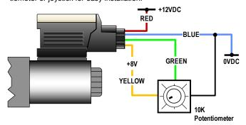
Ensure external signal source 0V is connected to same GND at this controller for correct operation
