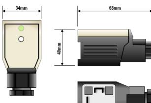
Controller interfaces with industry standard DIN 43650 - 3 pin connector as shown
