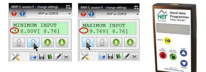
Use the up and down arrows to navigate through the parameter list. The display will show the next parameter in the list when pressed. The parameter name is on the first line and the value is on the second line. The list scrolls, stepping down from the last parameter to the first and vice-versa.
