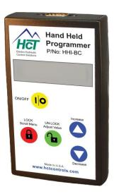
Use the up and down arrows to navigate through the parameter list. The display will show the next parameter in the list when pressed. The parameter name is on the first line and the value is on the second line. The list scrolls, stepping down from the last parameter to the first and vice-versa.
