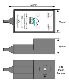
There are two indicator LEDs: STATUS and OUTPUT. The STATUS LED is green when the applied voltage is within the operating range.
