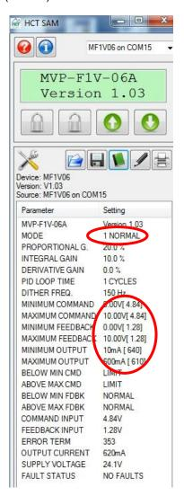
When command (1.04V) is less than the feedback (1.32V), the MVP-F will output 0 current.
