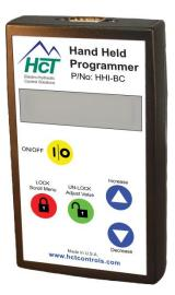
Use the up and down arrows to navigate through the parameter list. The display will show the next parameter in the list when pressed. The parameter name is on the first line and the value is on the second line. The list scrolls, stepping down from the last parameter to the first and vice-versa.
