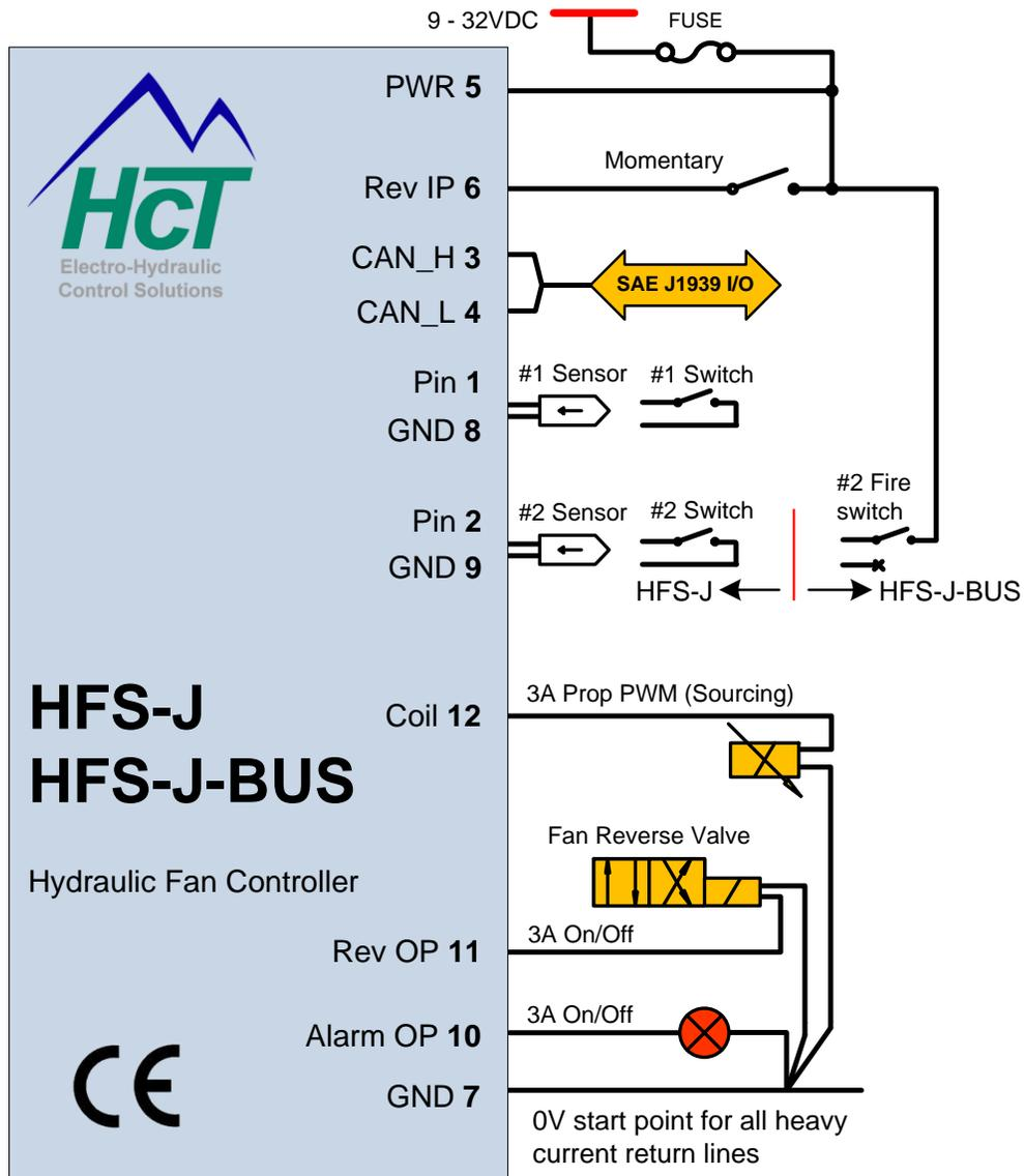
J1939 inputs - Charge air T, Transmission oil T, Engine coolant T, Engine RPM.
