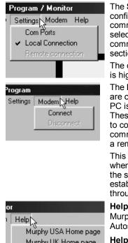
The **Settings** menu allows configuration of the PC RS232 communication port, and the selection of 'local' or 'remote' communication mode (see section 3.4 below).
