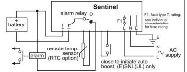
Note: battery output is isolated from chassis.
