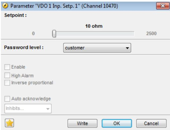
Adjust the resistance of the RMI sensor at the specific measuring value. In the example above the adjustment is 10 Ω at the engineering units minimum scale value.
