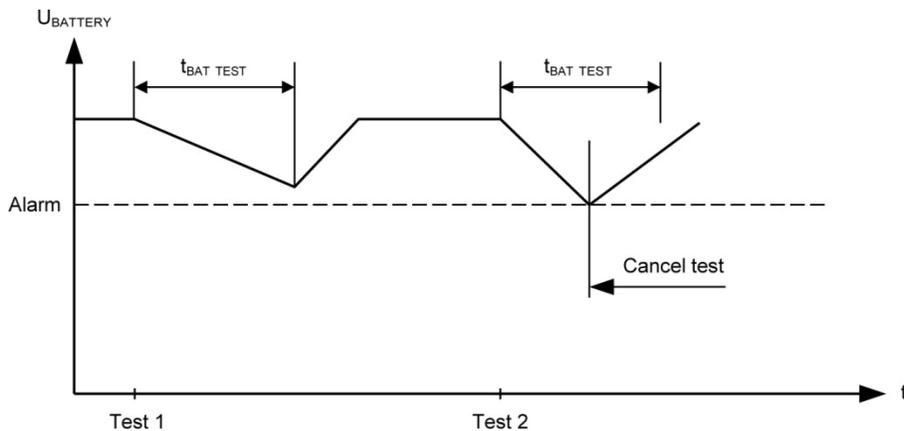
The drawing shows that test #1 is carried out without a large voltage drop of the battery voltage, whereas test #2 reaches the alarm set point.
