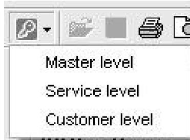
If the password level is not entered, it is not possible to enter the parameters.
