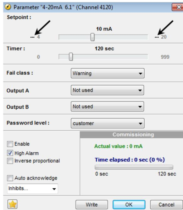
4. Adjust the input as required, for example, 0-5 bar. The display will then show 0 at 4 mA.
