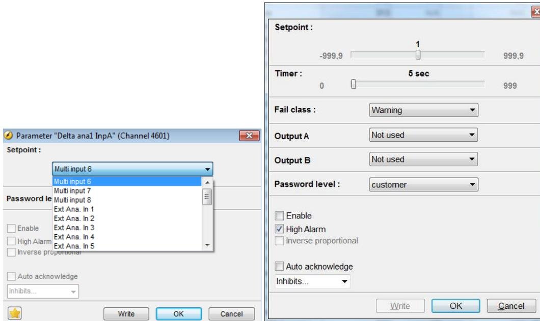
Two levels of alarms can be made of each differential measurement between sensor A and B.
