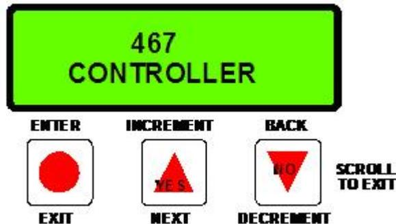
For example, if the controller receives a remote start signal, it will auto start the engine and display the current operation on the screen. These states include Crank On, Crank Off, Warm-up, Cooldown, etc. When the controller has brought the engine on stream, the display will scroll vertically through the engine vital signs. These include Oil Pressure, Engine Temperature, Engine Speed, Running Hours, etc.
