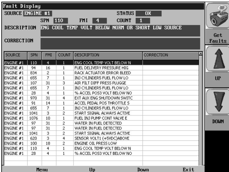
The following is a list of field definitions contained on the ENGINE DIAGNOSTICS screen:
