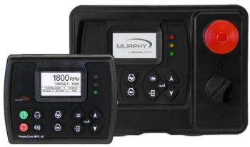
units, please download the latest PowerVision for Controllers configuration tool (**2.8.10599**), and load the new firmware including bootloader (**2.8.10024**) into your current controller. This may require additional Murphy equipment such as the MPC-10 USB programming harness or an ECOM communication dongle, which are available for purchase.
