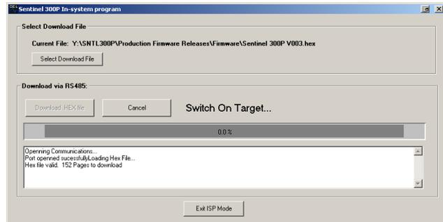
Whilst programming the **Charger Firmware** the LCD display, if connected, will cycle through reporting COMS FAILURE and attempts to restart until programming is completed and charger resets.
