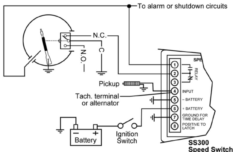
**NOTE:** Relay contacts transfer above speed setting after 4 seconds delay for idle and running speed oil pressure.
