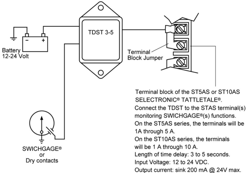
Terminal block of the ST5AS or ST10AS SELECTRONIC® TATTLETALE®. Connect the TDST to the STAS terminal(s) monitoring SWICHGAGE®(s) functions. On the ST5AS series, the terminals will be 1A through 5 A. On the ST10AS series, the terminals will be 1 A through 10 A. Length of time delay: 3 to 5 seconds. Input Voltage: 12 to 24 VDC. Output current: sink 200 mA @ 24V max.
