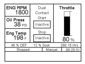
The screen above displays the auto start/stop type and illustrates the throttling method for the auto start/stop. This screen is a default setting which displays dual contact start (floats) and auto throttle to a Running Loaded Speed. The percent shown below the bar is the percent between the minimum and maximum speed set in the controller under Engine Settings.
