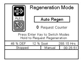
When selected to be shown, the screen above displays the Regeneration Control for Tier 4 engines. The setting to show this page is in the Tier 4 Menu within Engine Settings of the main menu. Use the Enter button to change from Auto to Inhibit. With Auto Regen selected, hold the Enter button for Regeneration request.
