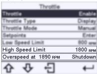
If Throttle is disabled, Overspeed type will be disabled automatically and when the Throttle is enabled, Overspeed shutdown type will be back to its previous setting.
