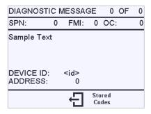
Press the and to scroll through additional messages if any are present. Each saved code shows the SPN (Suspect Parameter Number), FMI (Failure Mode Identifier) and OC (Occurrence Count). The OC indicates if the same fault occurred more than once. If available, a text explanation of the Warning or Shutdown and the Device ID Address also displays.
