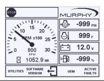
The ability to add shut-down set points is possible for Temperature and Pressure. By default they are disabled. When changing from Electronic to Mechanical engines, all Resistive Inputs will be defaulted to Murphy senders and respective shutdowns will be enabled. When going from Mechanical to Electronic, all Resistive Inputs will be disabled by default.
