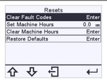
Clear Fault Codes: To clear existing Fault Codes, press while highlighting this selection. A **Request Sent to Clear Faults** message will display.
