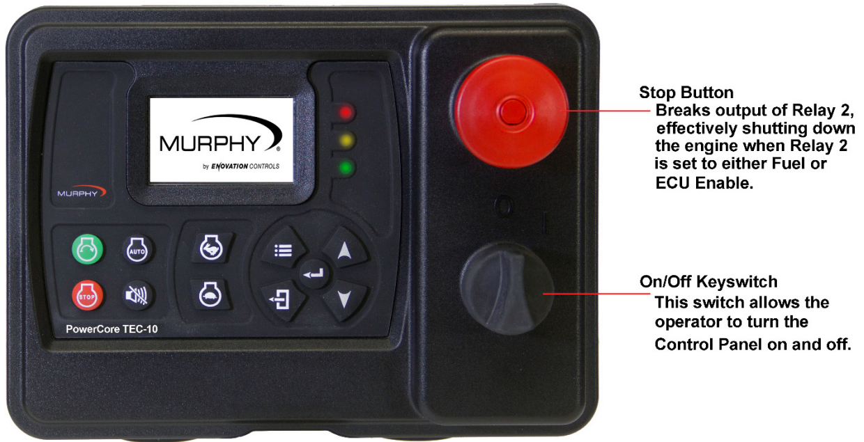
Figure 2: Panel stop button and on/off keyswitch
