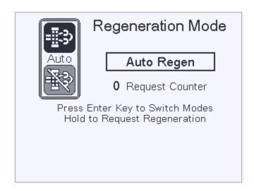
This screen displays the Regeneration Control for Tier 4 engines. Use the Enter button to change from Auto to Inhibit. With Auto Regen selected, hold the Enter button for Regeneration request.
