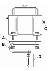
3. The hardened set screw and nuts **(D)** are used to tighten the switch to an I-Beam or cross member such as a Sampson post of an oil well pump jack.
