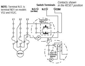
VS2, VS2C, VS2EX, VS2EXR, VS2EXRB and VS94 Typical Wiring Diagram for Distributor Ignition or Diesel
