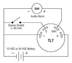
NOTE: Typical wiring with negative ground. Although designed to be used with Murphy Swichgage, the TL7 can be used with any dry contact type switch.
