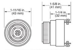
Mounting Hole: 1-1/8 in. (29 mm) diameter Maximum Panel Thickness: 1/8 in. (3 mm)
