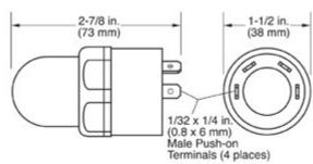
Mounting Hole: 1-1/8 in. (29 mm) diameter Maximum Panel Thickness: 1/4 in. (6 mm)
